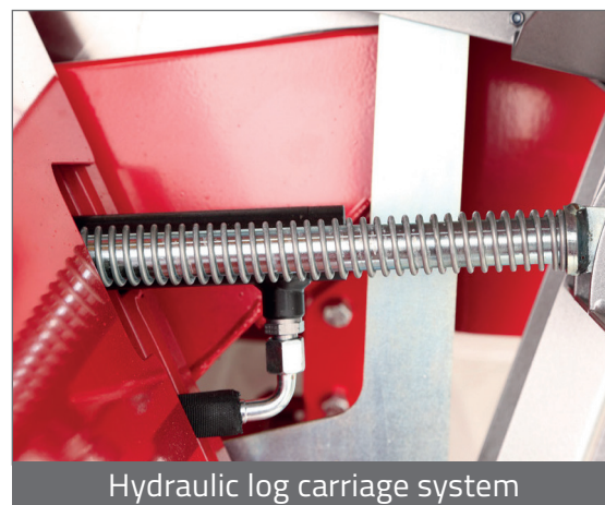
Valve and speed regulation for log carriage
