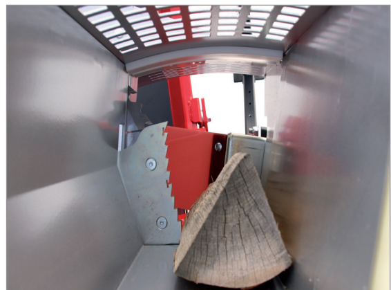
Log grip system locks the wood while sawing
