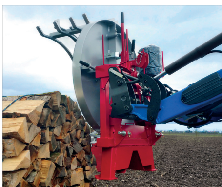
Bundler with polyester strips mechanical pivoting on 3-points hitch + euro linkage for front loader
