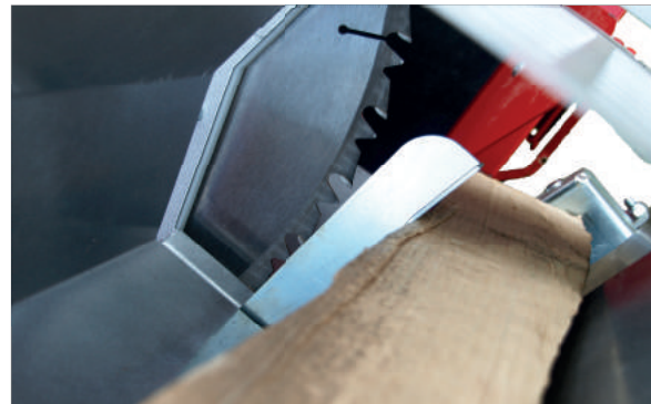
Log grip system that locks the wood while sawing
