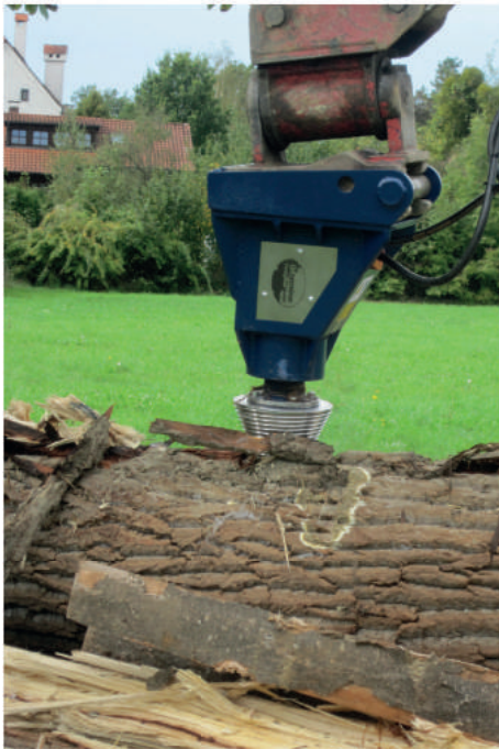
Ø200mm cone (double-edged thread) for KB 800 and KB-S 800
